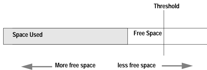
Figure 21-1: Log segment with a last-chance threshold
